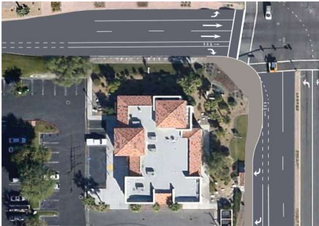
Figure 28: Typical Right-turn Departure NEV-Bike Lane
